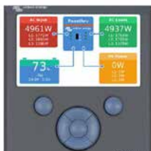
Color Control GX, showing a PV application
